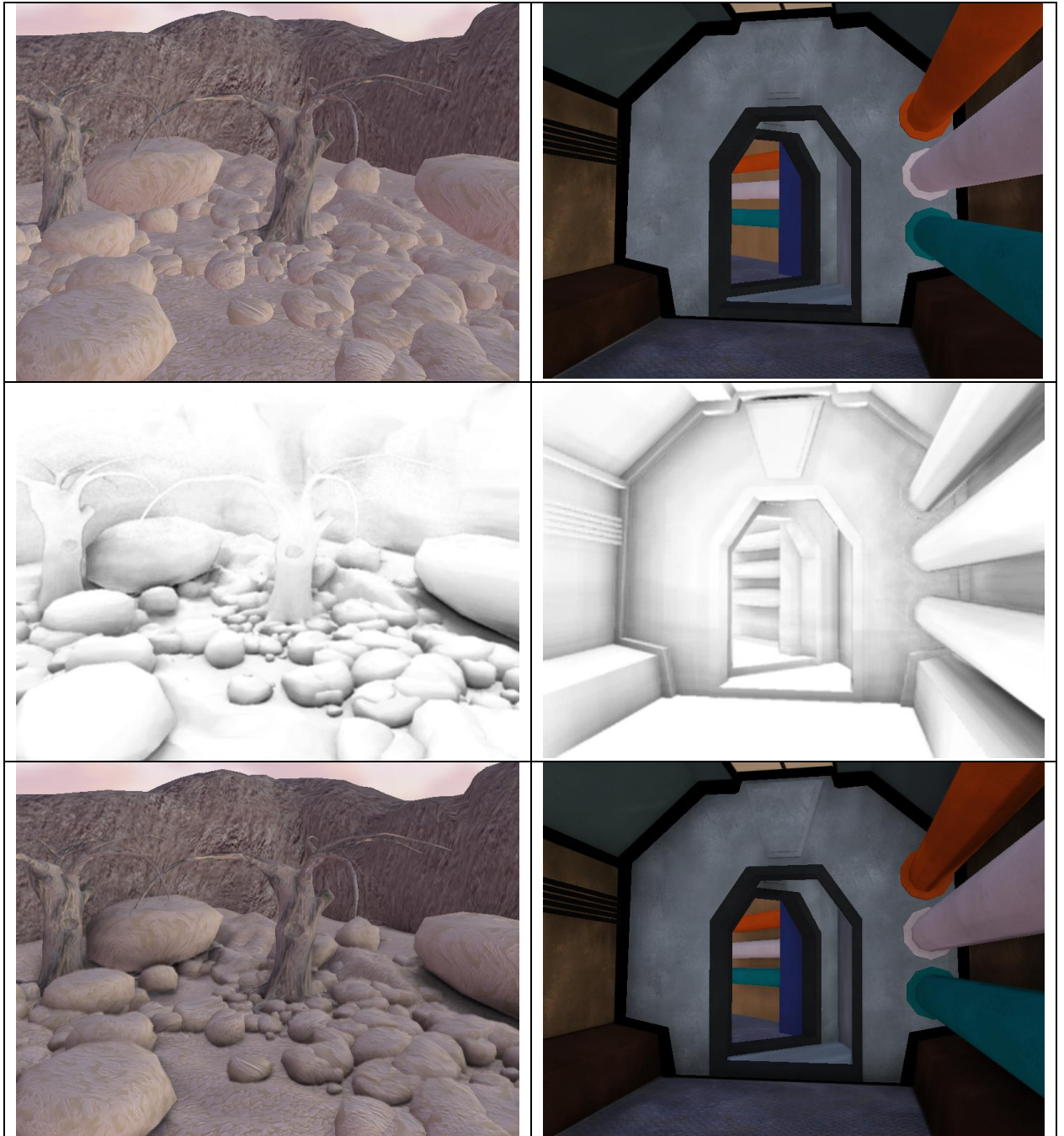
Figure 6. The Rocky Scene and the Space Station Scene rendered with classical ambient reflection model a(\bar{x})L^a (top row), obscurances only (middle row), and using the obscurances reflection model a(\bar{x})W(\bar{x})L^a . The obscurances values are generated from 16 samples per pixel in real-time.
